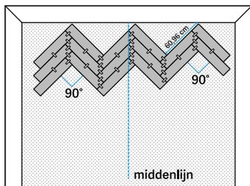
3. Lay the joined strips against the starting wall, with the points straight on the centre line.
