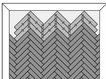
6. Repeat this procedure to the left and right of the laid starting strip. Continuously check that all angles are still 90°.
