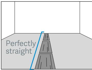
1. Glue the first measured and marked part according to the manufacturer's instructions. Observe the correct opening time and processing time. Place the mFLOR Dryback panels exactly along the perfectly straight starting line.
