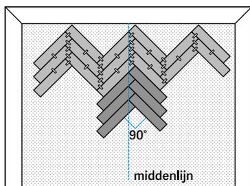
5. Apply glue to the floor across a width of two strips and lay these two strips on the glue. When doing so, carefully follow the glue manufacturer's instructions regarding opening time and application time.
