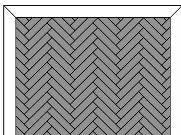
7. Remove the strips stuck together with tape and lay the floor close against the starting wall.
