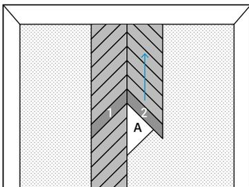
6. When the starting row is properly fixed, continue with the second row, to the right of the starting row. Start again with the starting strip, using guide piece A. Again, work first upwards and only then downwards.
