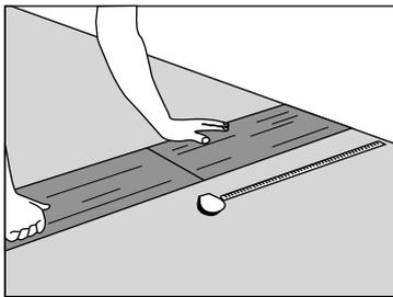
3. Measure the last panel of the first row carefully and place it without stress against the wall or skirting.
