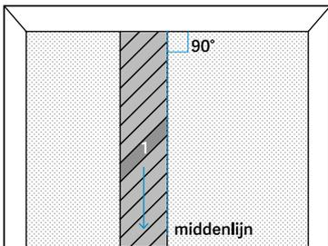
4. Remove guide piece A and apply glue to the floor below the starting strip. Then lay the strips below the starting strip on the glue.
