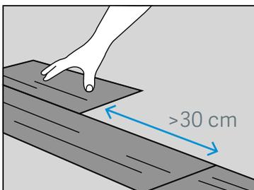
5. For the second and each subsequent row, take a new panel and decide how large the panel should be (or use a piece left over from one of the previous rows). With boards, make sure that the joint of the short side is at least 30 cm from the joint of the short side of the previous row; and at least 20 cm in the case of tiles.
