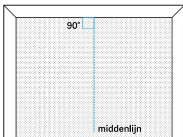
1. Identify the centre of the room (viewed from the starting wall) and make a line at right angles to the starting wall using a chalk line. This is the centre line.
