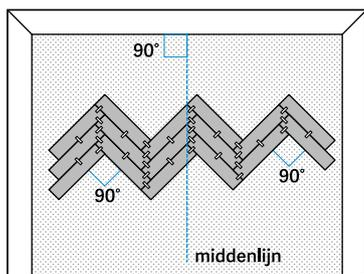
2. Lay two or three rows of strips against each other. Make sure that the corners are exactly 90° and fasten the strips tightly together with tape.
