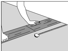
3. Measure the last panel of the first row carefully and place it without stress against the wall or plinth.
