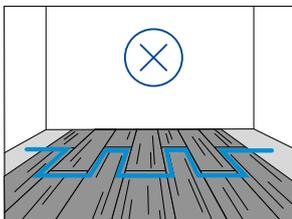
4. For a natural look, we recommend that the piece left over from the first row should not be used as the first piece of the second row. Avoid having a recognisable, repeating distance between the panels, which creates a kind of staircase effect. Boards are installed randomly and tiles can be installed in a straight line, in a half-brick bond or in an irregular bond.
