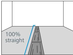
1. Glue the first part, measured and marked out, according to the manufacturer's instructions. Use the correct opening time and processing time. Place the mFLOR® dryback panels exactly along the perfectly straight starting line.
