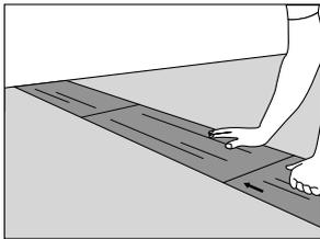
2. Lay the panels without stress and continuously against each other, taking into account the direction of the arrows on the backing in the case of large tiles.
