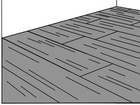
7. Cut the last row along the wall or any obstacles by measuring accurately or using contour jigs.
