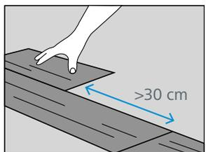
5. For the second and each subsequent row, take a new panel and decide how large the panel should be (or use a piece that is left over from one of the previous rows). Ensure that the joint of the short side is at least 30 cm from the joint of the short side of the previous row.
