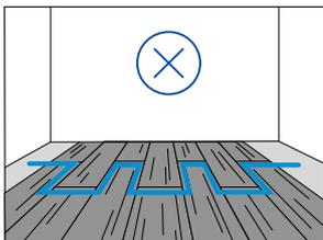
4. For a natural look, we recommend that the piece left over from the first row should not be used as the first piece of the second row. Avoid having a recognisable, repeating distance between the panels, which creates a kind of staircase effect.
