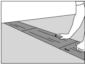
2. Following the direction of the arrows on the backing, lay the panels without stress and continuously against each other and against the wall or plinth.
